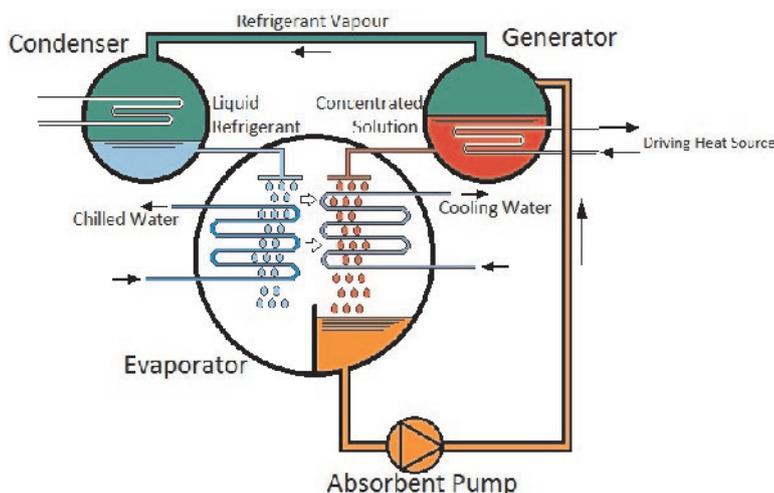
Figure 5: Schematic of an adsorption chiller.
