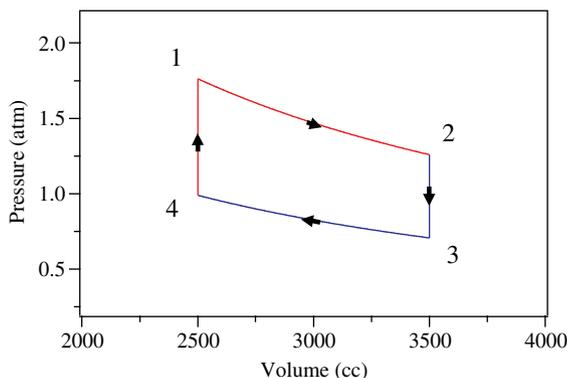
2. *Isovolumetric or Isochoric (constant volume) heat removal, 2 to 3.* The gas is passed through the regenerator, where it cools by transferring heat to the regenerator for use in the next cycle.
