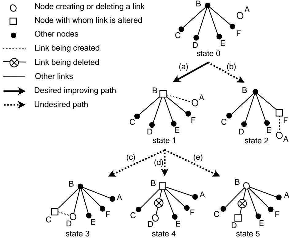
Figure 2: Directing Network Evolution for the Formation of Star Topology
